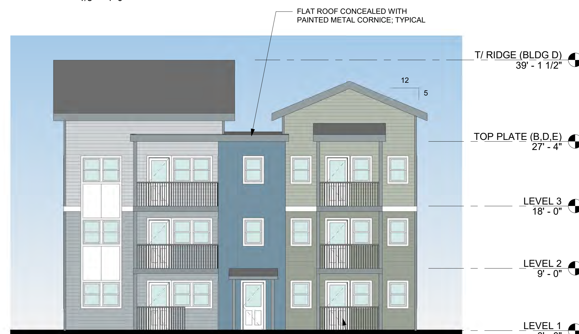
① BUILDING D - EAST ELEVATION (FROM COURTYARD) 1/8" = 1'-0"
