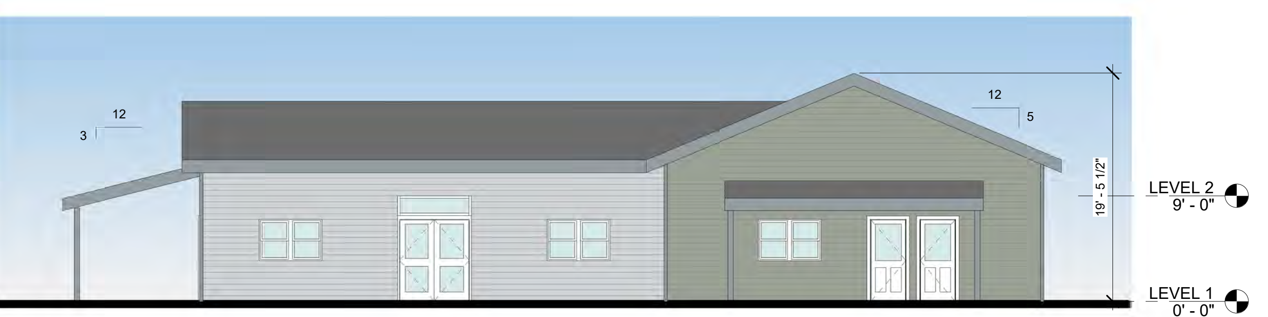
5 COMMUNITY BUILDING - SOUTH ELEVATION (FROM ALLEY) 1/8" = 1'-0"
