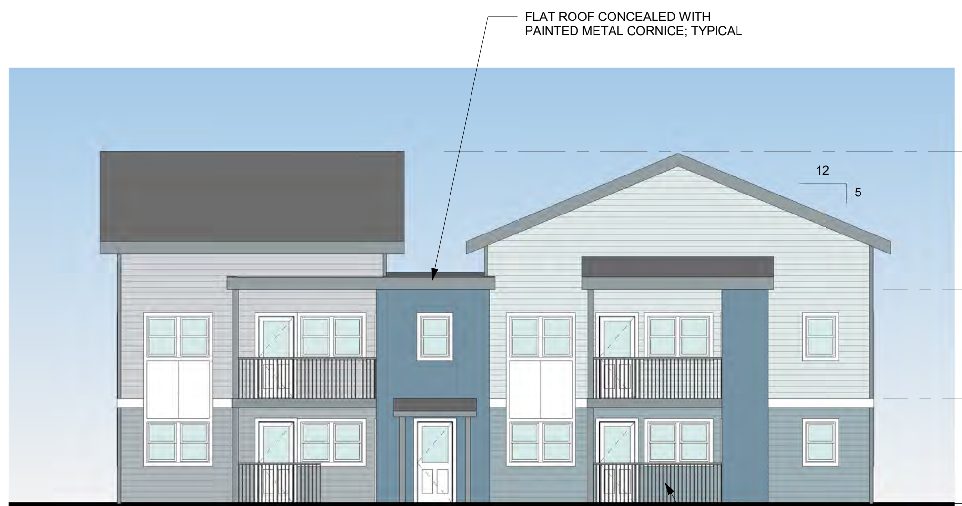
BUILDING A - EAST ELEVATION (FROM COURTYARD) 1/8" = 1'-0"
