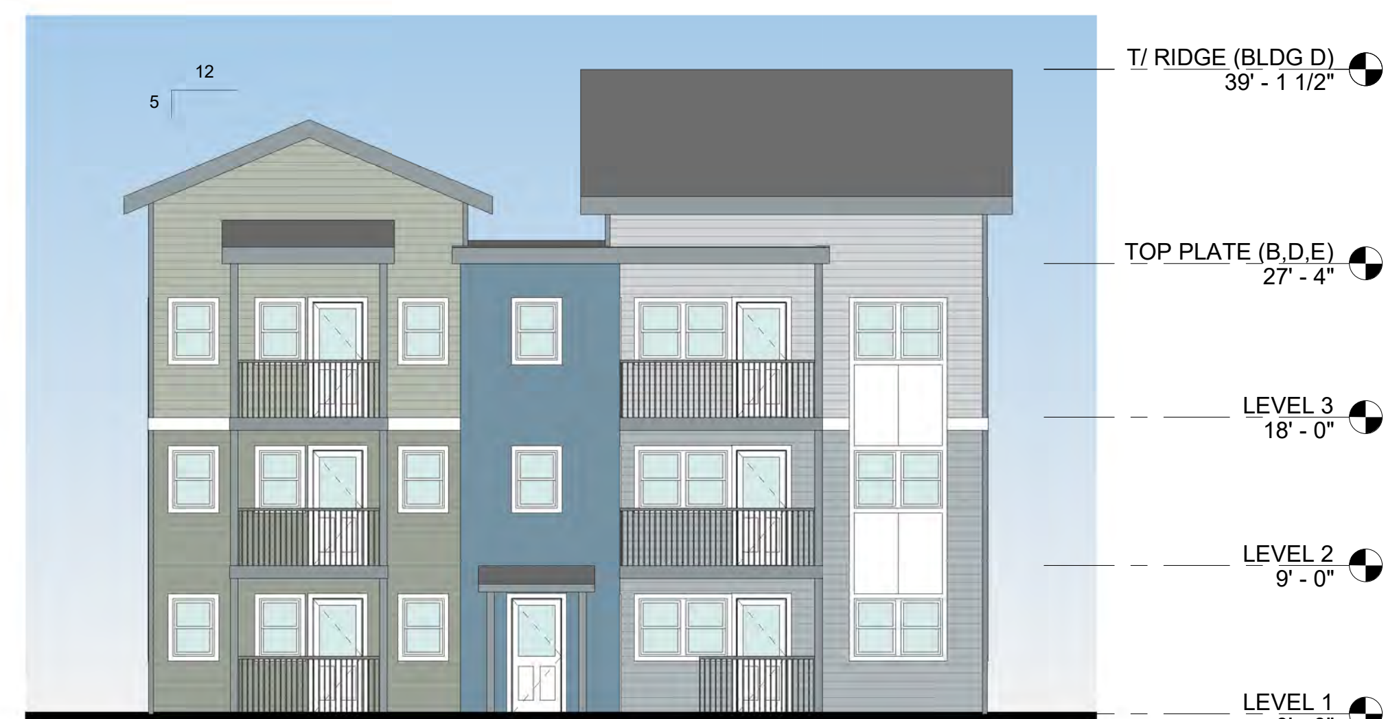
BUILDING E - WEST ELEVATION (FROM ① COURTYARD) 1/8" = 1'-0"
