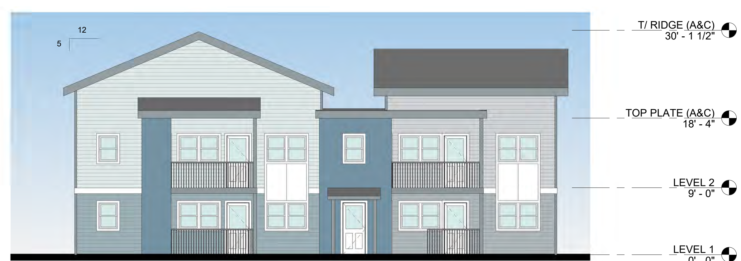
① BUILDING C - WEST ELEVATION (FROM COURTYARD) 1/8" = 1'-0"
