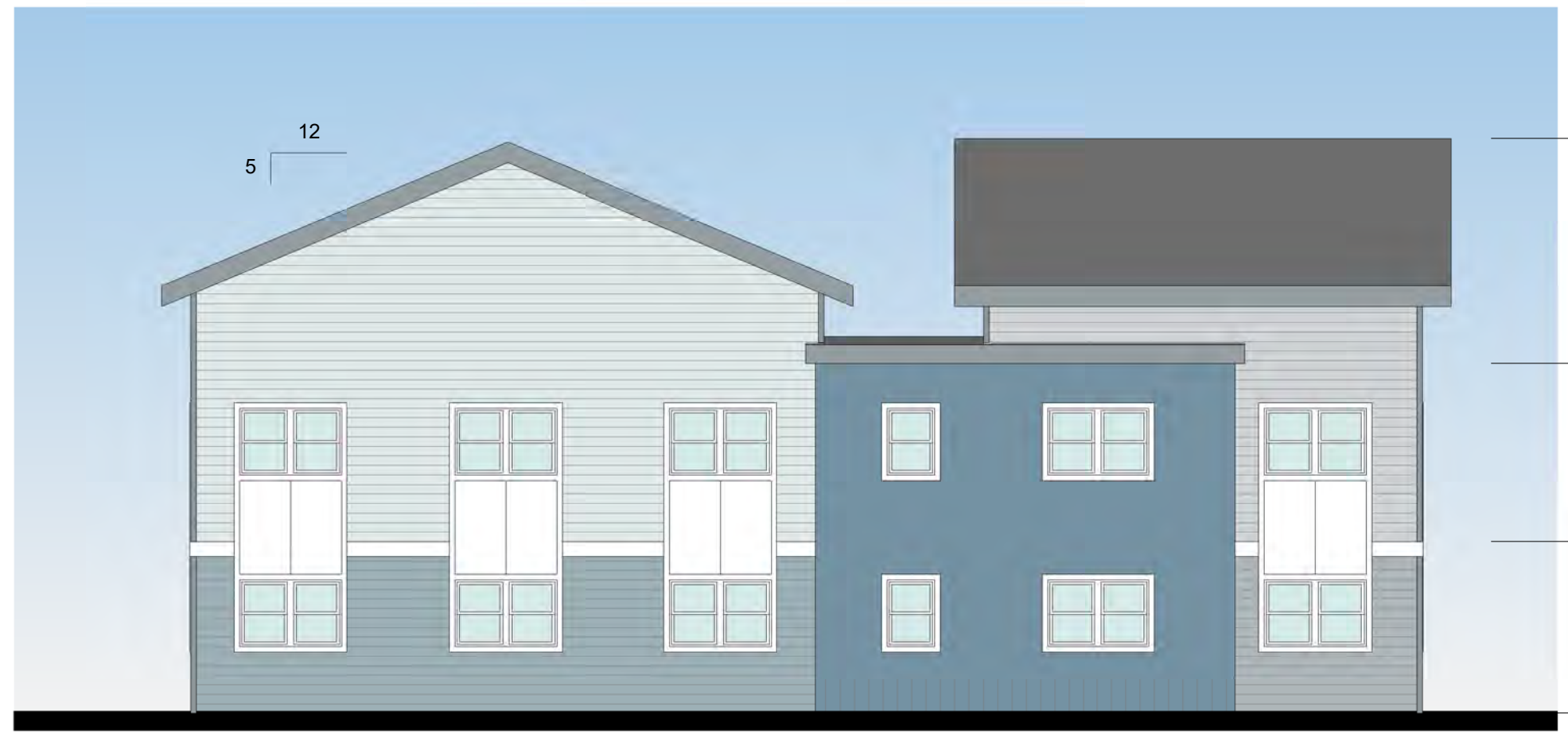
BUILDING A - WEST ELEVATION (FROM FIR STREET) 1/8" = 1'-0"
