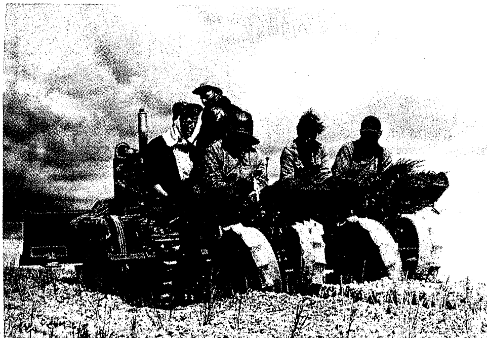
Figure 13. Machine planting of European beachgrass in open dune area.
