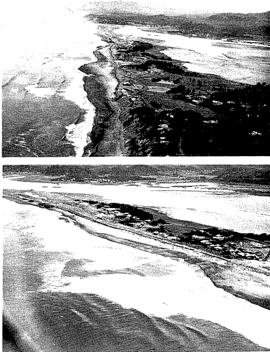
Figure 26. Embayments cut out of the beach and into the foredunes on Siletz Spit leading to property losses during December 1972 and January 1973, produced by seaward flowing rip currents (from Komar and Rea, 1976).
