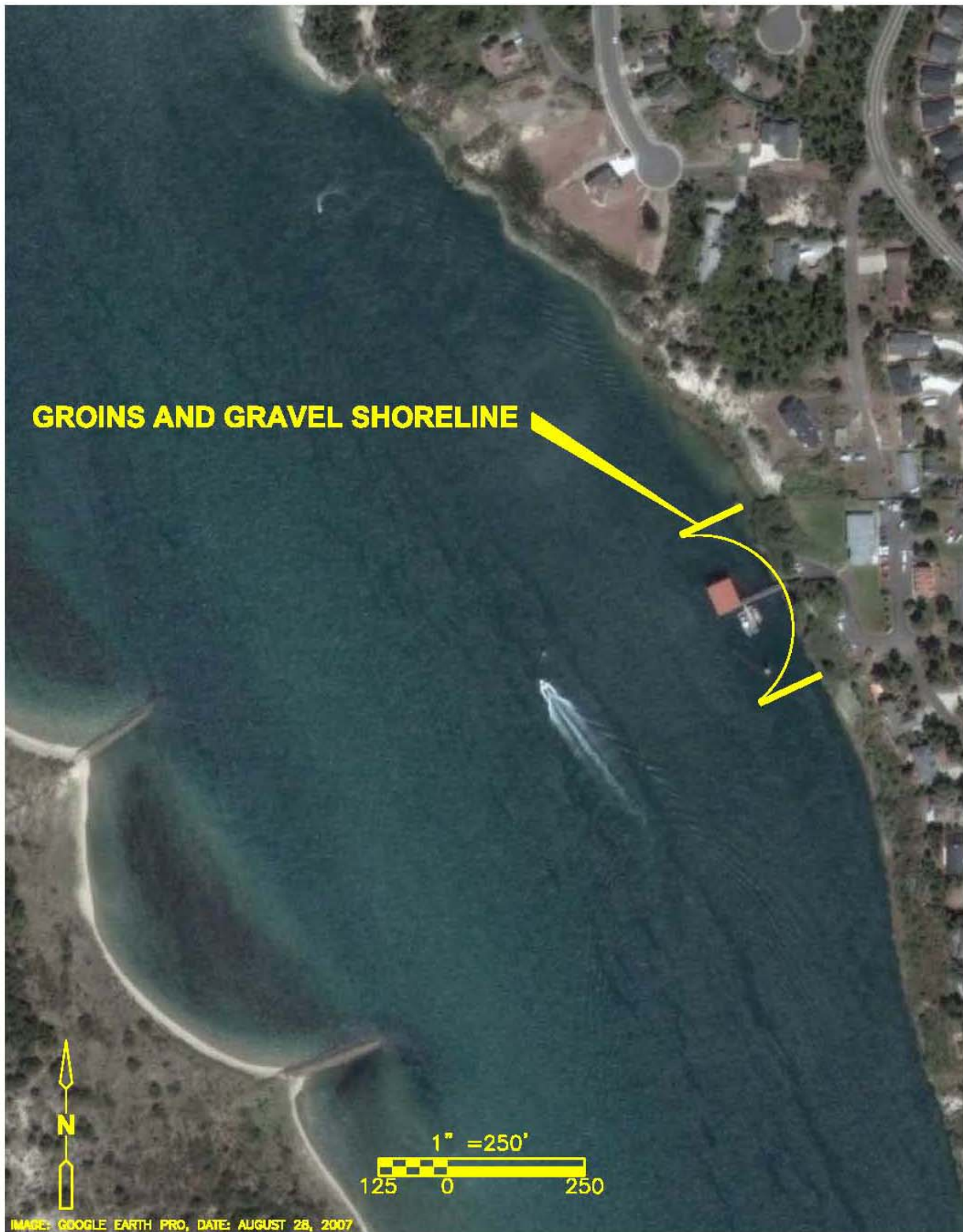
Figure 9. Action Alternative 1 - Construct Groins with Gravel Shoreline.
