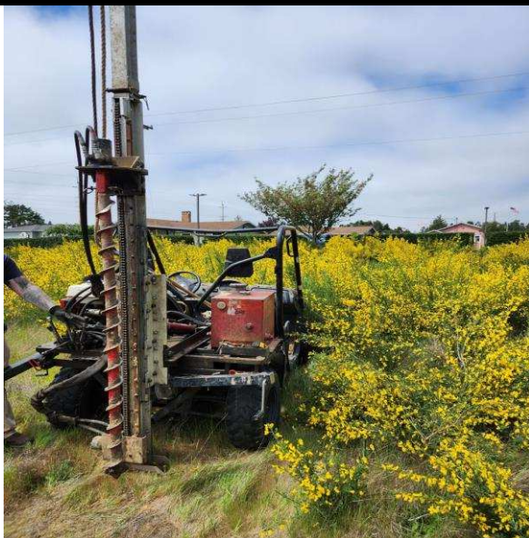
ATV mounted drill rig used for borings
