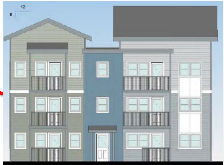
BUILDING E - WEST ELEVATION (FROM ① COURTYARD) 1/8" = 1'-0"
