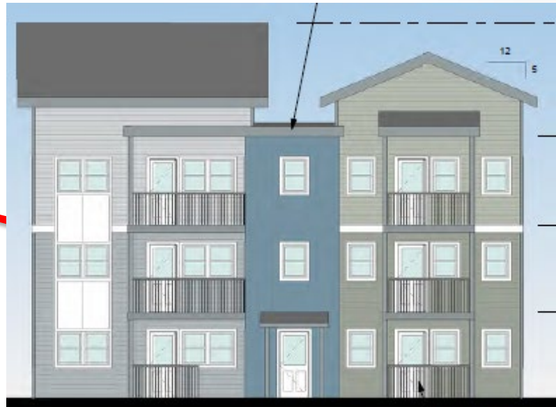
BUILDING D - EAST ELEVATION (FROM COURTYARD) ① 1/8" = 1'-0" STEEL RAILING POWR COATED GRAY; TYPIC
