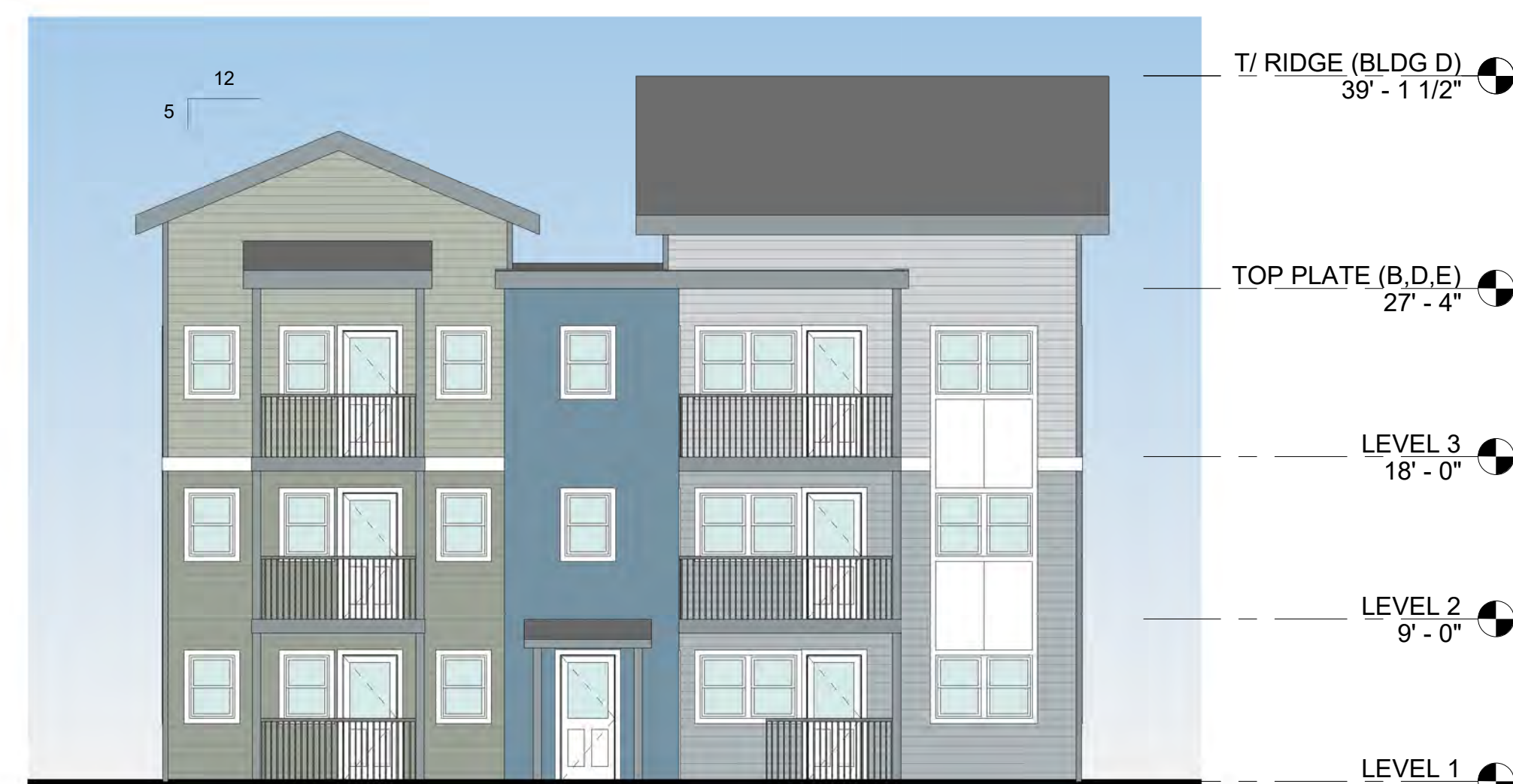
BUILDING E - WEST ELEVATION (FROM ① COURTYARD) 1/8" = 1'-0"
