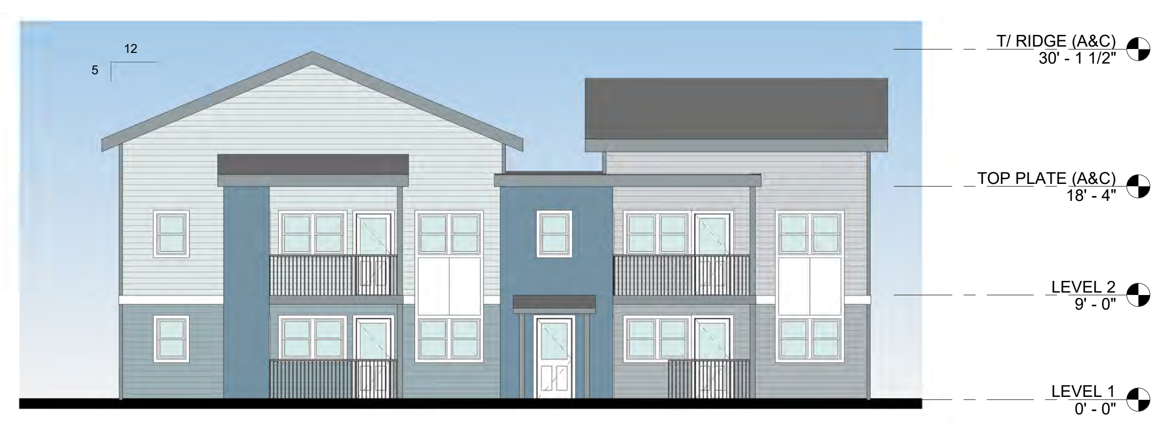
① BUILDING C - WEST ELEVATION (FROM COURTYARD) 1/8" = 1'-0"
