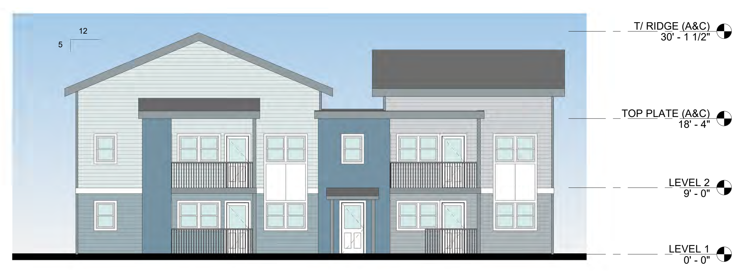
① BUILDING C - WEST ELEVATION (FROM COURTYARD) 1/8" = 1'-0"
