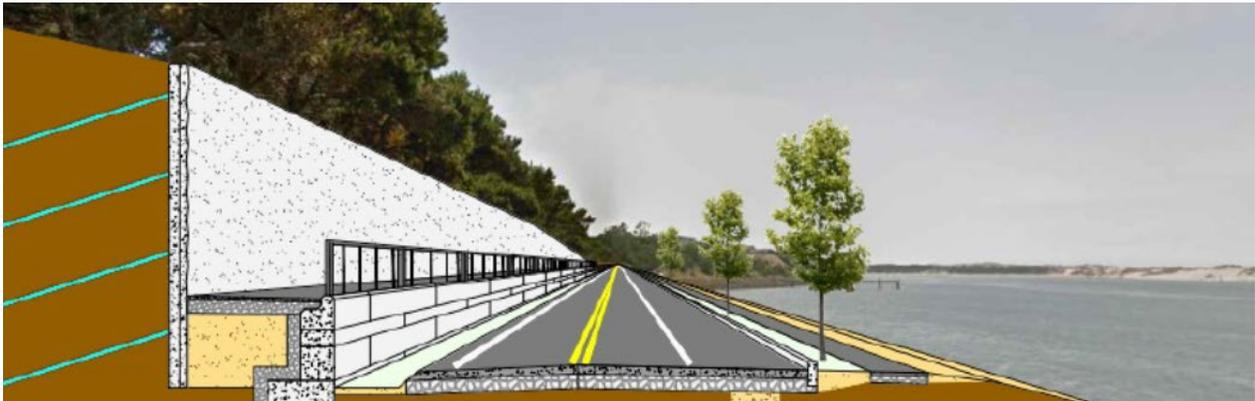
One of the key features of the project is dealing with the slopes on the east side of Rhododendron Drive south of New Hope Lane. The project utilizes the slope to the benefit of the project by incorporating the multi-use path and elevating it in this section of the project. This will allow pedestrians and bicyclists a view of the river and sand dunes from above motor vehicle level.
