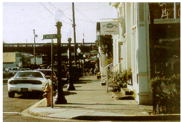
On-street parking, curbside zone, walking lane and storefront zone are essential elements of a mainstreet.
